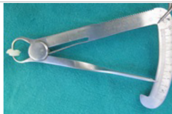
Figure 11: Measurement of the Restoration Thickness at 2mm from the Groove
