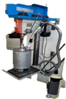
Figure 4: Procedure for collection of nanoparticles of iron through the dry mill of high energy (Source: own production)(Unpublished photo)
