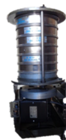
Figure 3: Machine vibrating sieve for the selection of the size of particles of iron.(source: own production)(Unpublished photo).
