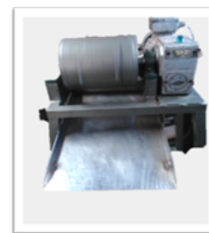
Figure 2: Grinding of chip of iron cast in a pellet mill / (source: own production)(Unpublished photo)
