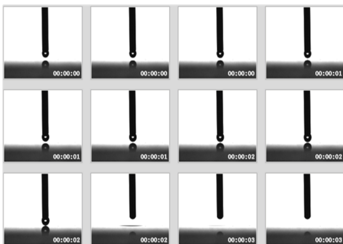
Figure 4: Still images captured from video recordings for a water droplet (3 μL) spreading on a substrate covered with superhydrophilic, anti-fogging and antireflective coatings.
