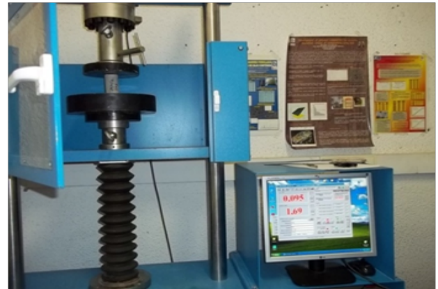
Figure 2: Press used for compression and tensile strength tests. Source: Department of Materials Science and Metallurgical Engineering, UB.
