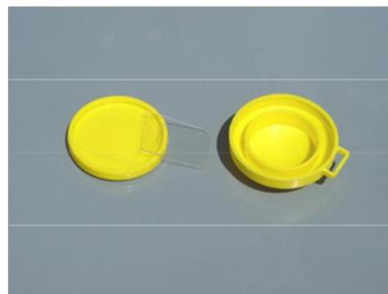
Figure 1: Disassembled dosimeter cartridge type NRPB with detector CR-39
