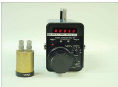
**Figure 2:** RDA-200 Meter (Pylon, Canada) for grab sampling
