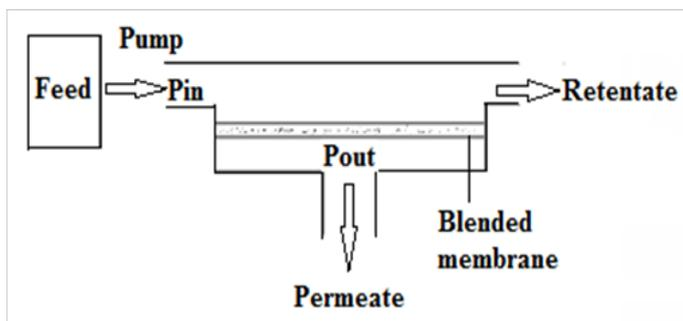
**Figure 1:** Cross flow filtration module design
