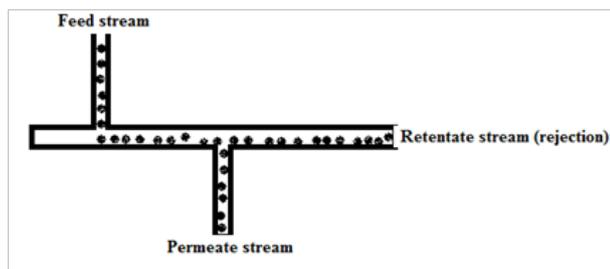
**Figure 3:** Simplified 2D geometry of the flow domain.
