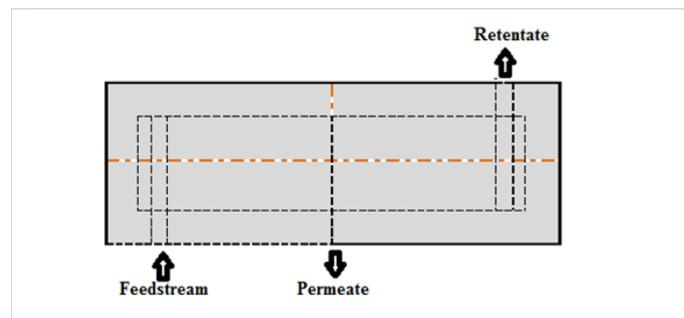
**Figure 2:** Geometry of cross flow filtration design.
